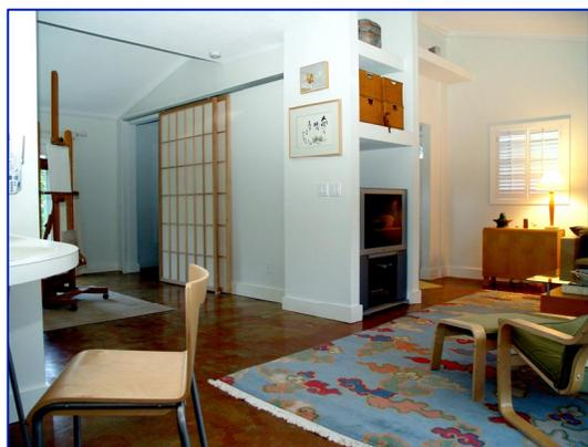
The Home Front, Inc. SIP houses have vaulted ceilings and ductwork inside the conditioned space. (Source: Home Front, Inc.)
